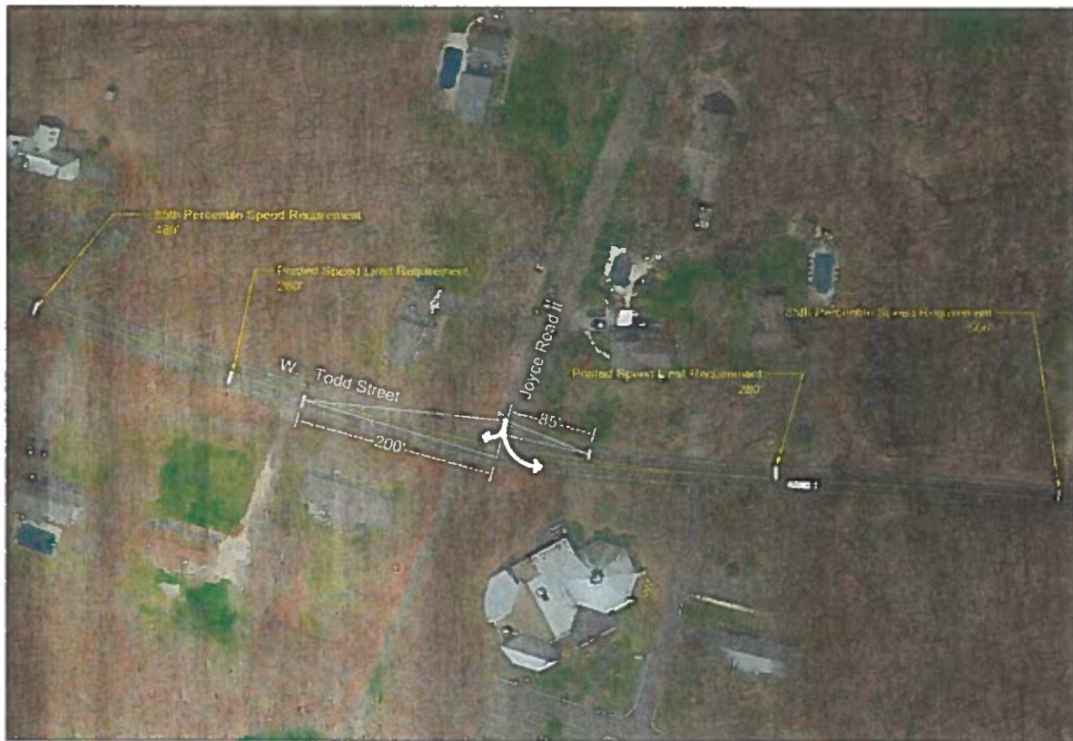
Figure 5- Existing and Required Intersection Sight Distance
