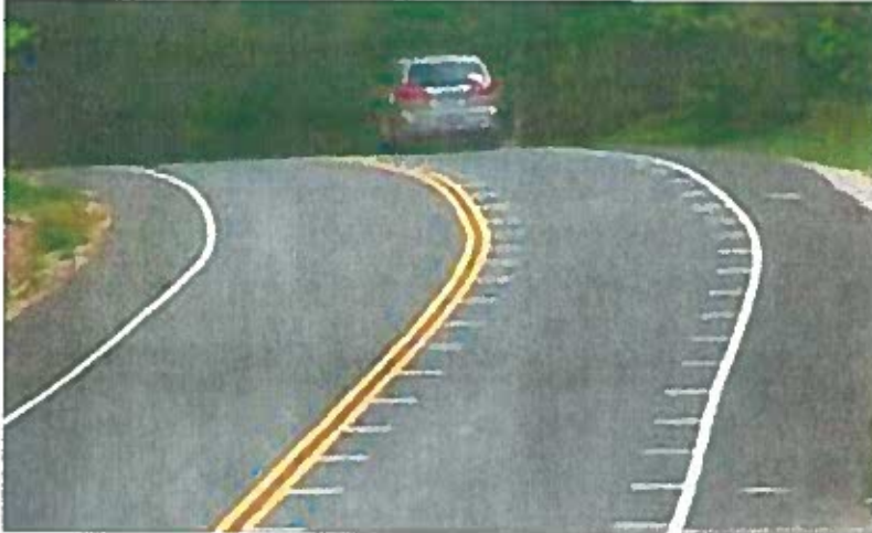
Figure 9- Transverse Pavement Marking
